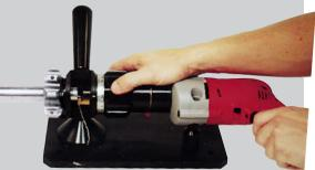
An optional mounting base is available to quickly convert the hand held machine to a bench mounted system.
